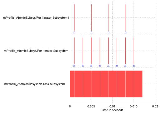
Plot of recorded profiling data over 0.016999 seconds
