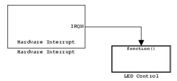
In this model, the Hardware Interrupt block installs a task that runs when it detects an external interrupt. This task then performs the specified operation.
