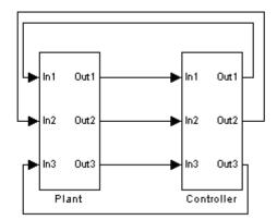
Your starting point in developing a combined plant and controller system model is to model the combined system as two subsystems in closed-loop simulation. As your design progresses, you can use Simulink external mode with standard Real-Time Workshop targets (such as GRT or ERT) to help you model the controller system separately from the plant.
