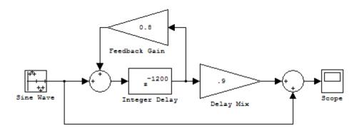
Look for the Integer Delay block in the Discrete library of Simulink and the Gain block in the Commonly Used Blocks library. This model implements an audio signal reverberation scheme. Part of the input audio signal passes directly to the output. A delayed version passes through a feedback loop before reaching the output. The result is an echo, or reverberation, added to the audio output.
