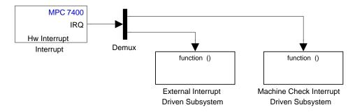
Here is the block mask showing the external and Machine check interrupts selected.
