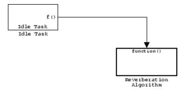
The function generated for this task normally runs in free-running mode—repetitively and indefinitely. However, the input and output blocks in this subsystem run in blocking mode. As a result, subsystem execution of the reverberation function is the same as the subsystem described for the Free-Running Task. Task execution is data driven via a background DMA interrupt-controlled ISR, shown in the following figure.
